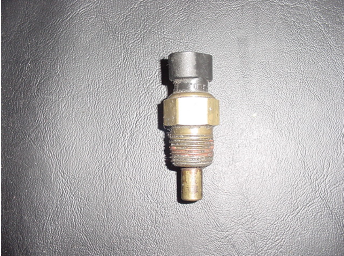
Coolant (oil) Temp sensor (Wells#SU109)
